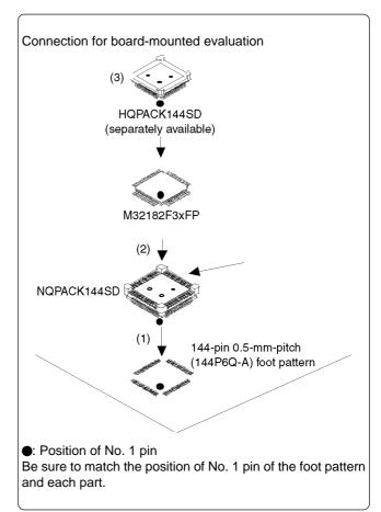
Figure 4 Connection for board-mounted evaluation
